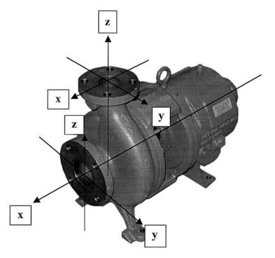
M<sub>xd</sub> max = allowable moment about x-axis on discharge nozzle  $M_{vd}$  max = allowable moment about y-axis on discharge nozzle  $M_{zd}$  max = allowable moment about z-axis on discharge nozzle
