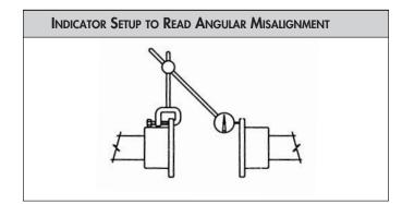
After each change, it is necessary to recheck both angular and offset alignment of the coupling. After driver is aligned to the pump, tighten all hold-down bolts and then recheck alignment.
