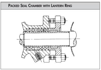
S = When soft packing rings are furnished in a set with metallic rings, install the soft rings in the locations marked "S".
