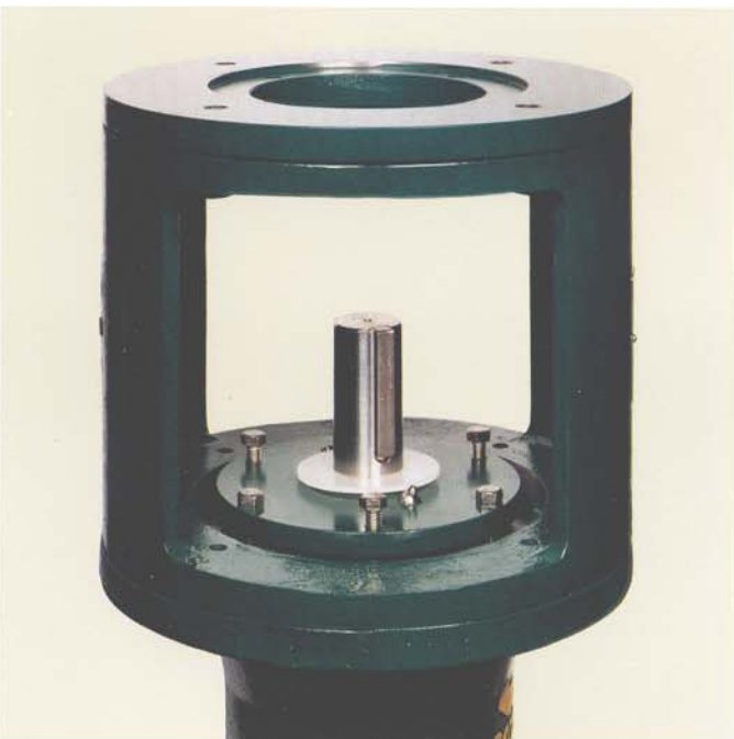
External impeller adjustment is accomplished with bearing housing jack screws
