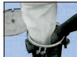
Remove filter bag from chamber.
