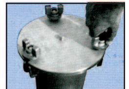
Drop in new bag. Replace bag holder and secure cover.
