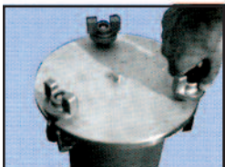
Unscrew 3 hand knobs and pivot knobs away from cover.
