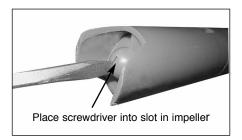
Now turn pump over and place screw driver into screwdriver slot in impeller (10). Unthread impeller (10) by turning it counter clockwise. Hold the 3/8" socket to prevent turning of the coupling nut (5).
