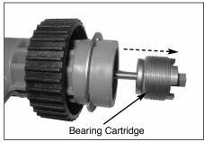
5. Using a small pair of pliers, grip the shaft (7) 2" below the bearing cartridge (11). Using a 3/8" wrench, unthread the coupling nut (5) counter clockwise. Once coupling nut (5) is unthreaded, simply slide the bearing cartridge (11) off the shaft (7). Vapor seal (3) can now slide upward off the shaft (7). Seal (3) should only be removed/installed upward. Check seal (3) for wear and replace if necessary.
